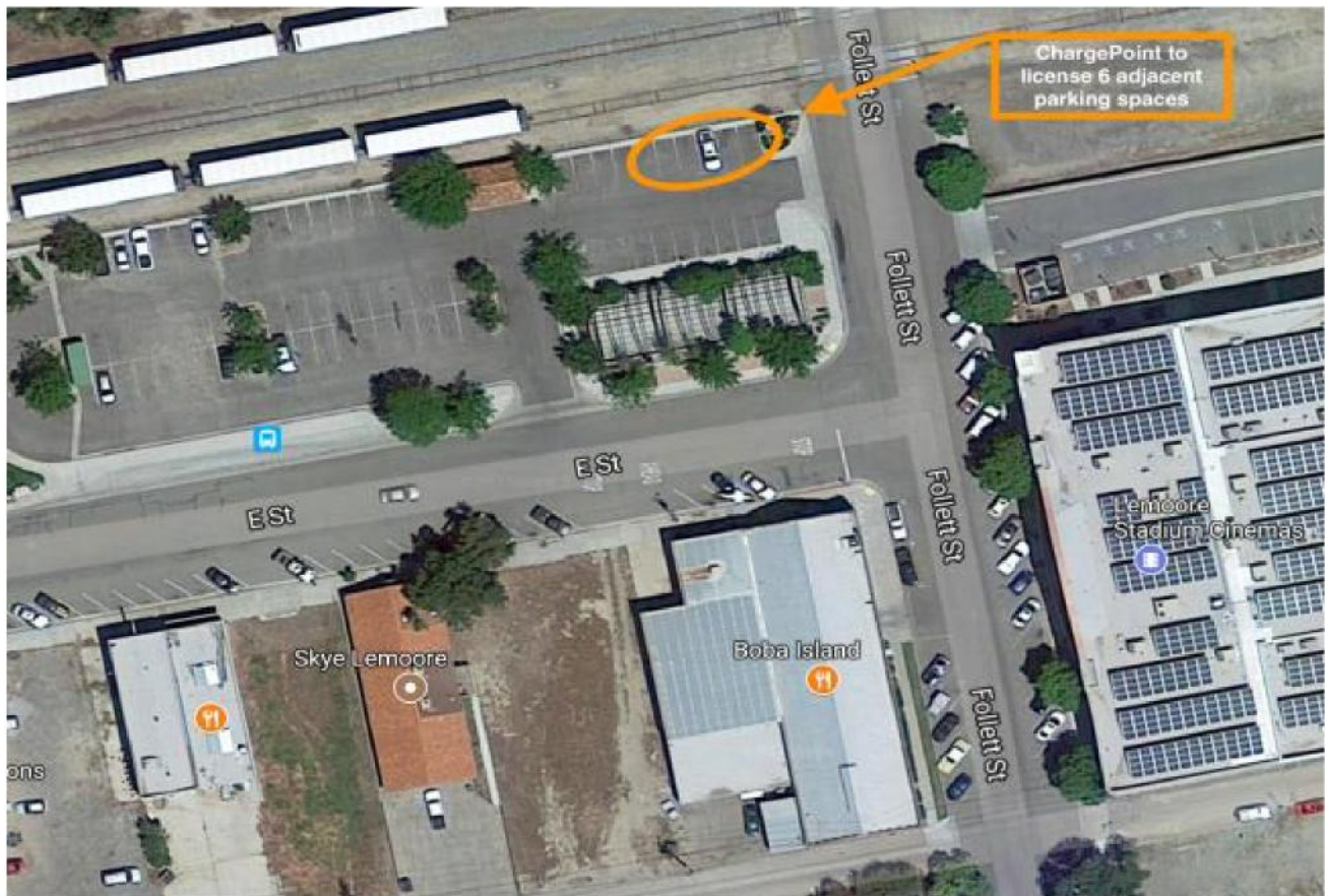
Figure A1 Parking lot site plan and picture above shows the location of the 6 parking spaces to be licensed and context for the planned section of the parking facility for the ChargePoint Express Plus equipment installation.
