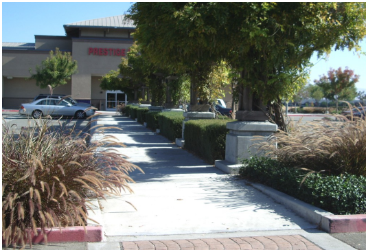
Desirable: A system of hard-surface internal walkways at least 4 feet wide that connect buildings to each other, to onsite automobile
