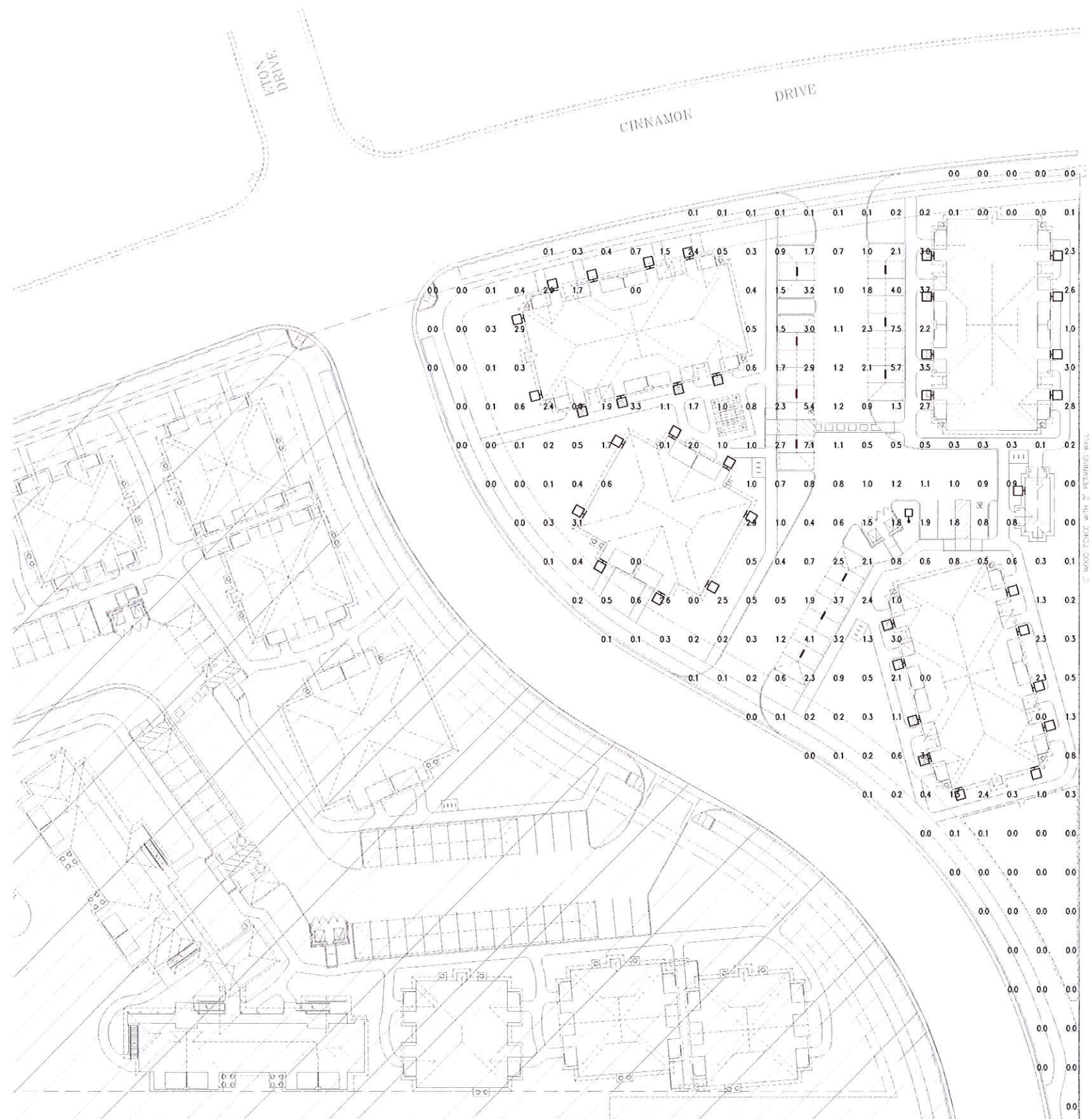
1 SITE PHOTOMETRIC PLAN SCALE: 1" = 30'-0" NORTH
